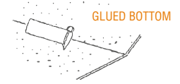
Place the dispenser on the adhesive base or hang the dispenser under the canopy by opening and closing the lid of the vial in such a way that the supporting wire of the trap remains in the eyelet of the lid.
